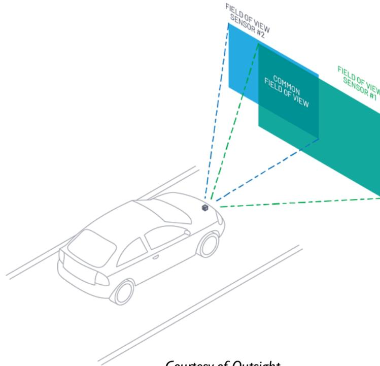
When sensors are positioned apart from each other, they will have a different perspective on the vehicle's environment (parallax) which may lead to a situation in which one sensor can perceive an object, while it is occluded for the other sensor
