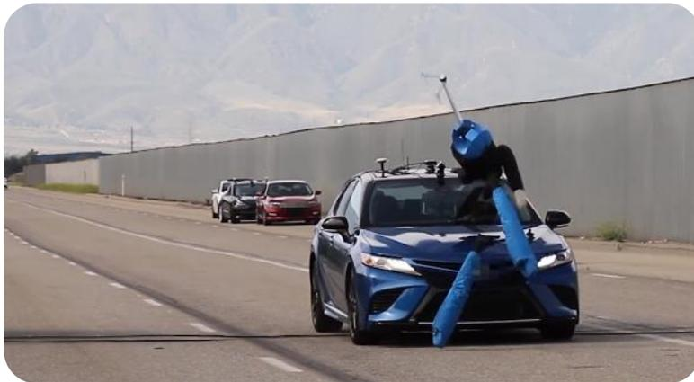
A dummy pedestrian struck by a vehicle during the test.
