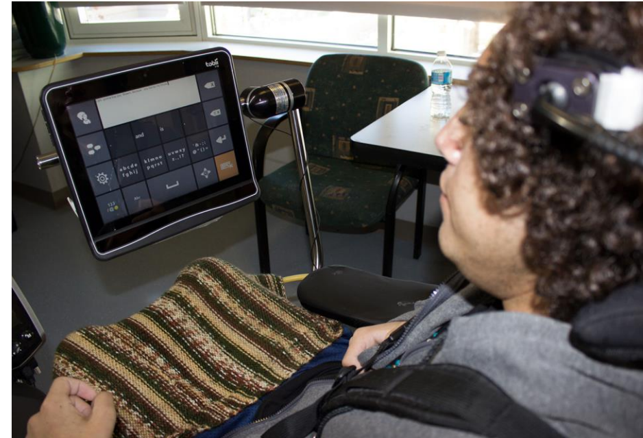
Tobii Assistive Technology. Eye interaction system with remote eye tracking integrated into a tablet
