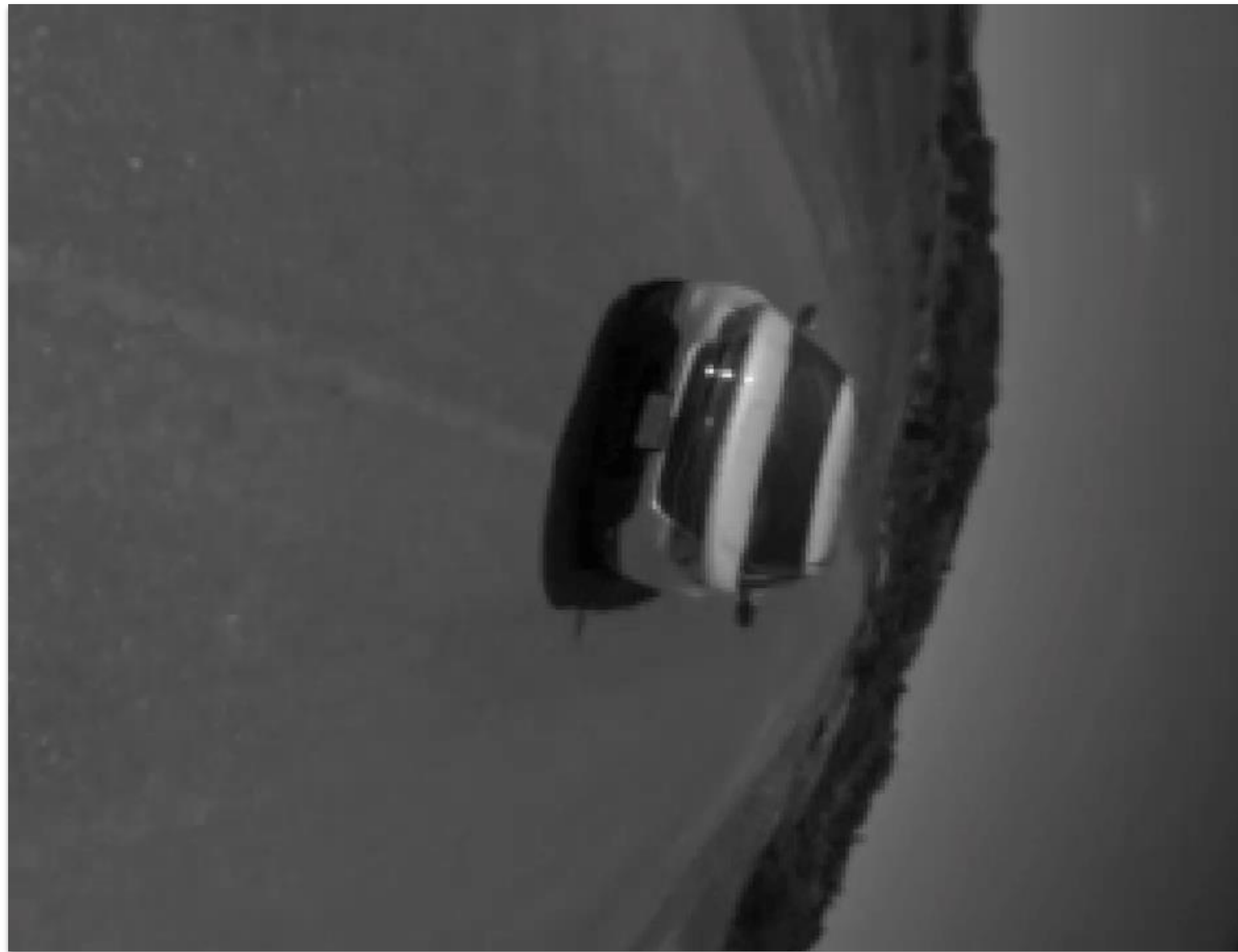
Rolling shutter deforms rigid objects like the horizon line and the vehicle itself.
