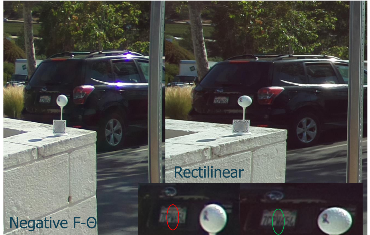
Two 90° HFoV lenses on IMX477. Left 10% of image is shown.
