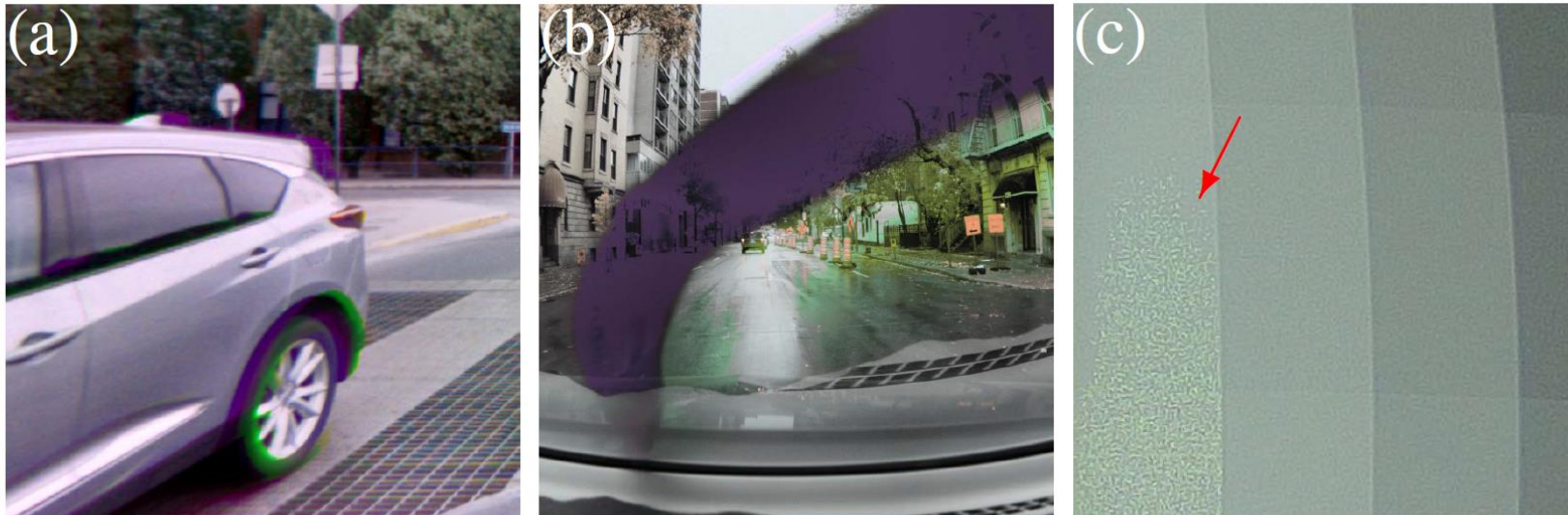
Figure 2: Common HDR multiplexing artifacts. Crops (a) and (b): ghosting. Crop (c): SNR discontinuity.
