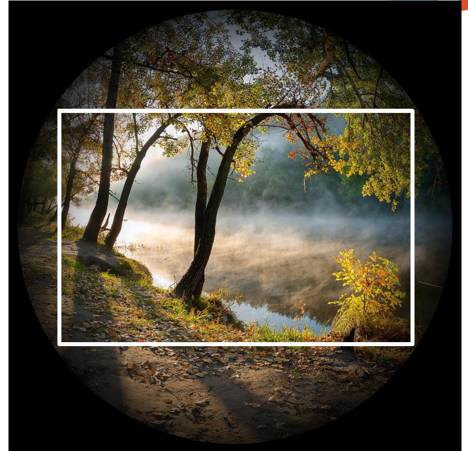
Illustration of image circle on sensor plane.
