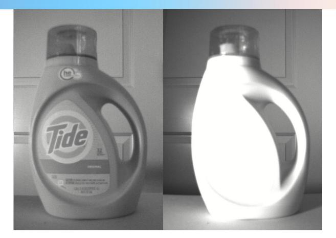
Infrared cameras and lighting allows seeing defects that visible light cameras can't.
