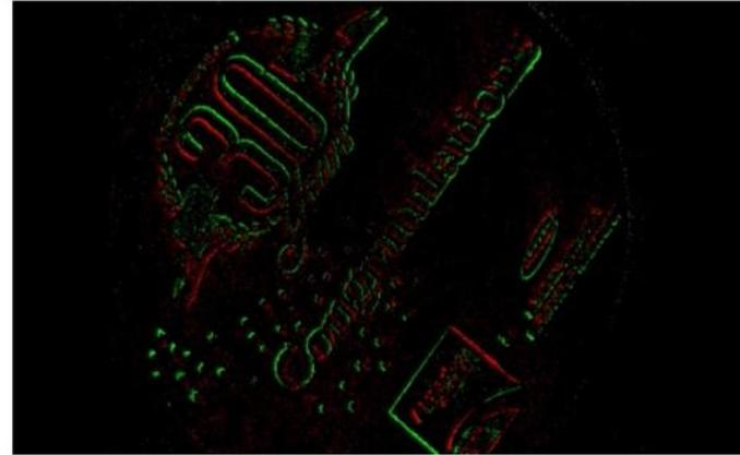
DVS image for rotating object (~220 rpm)
