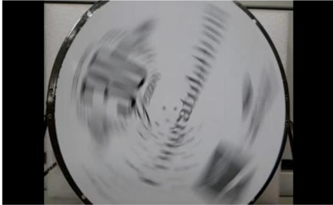
CIS image for rotating object (~220 rpm)
